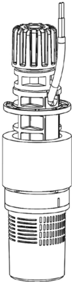
FILTO CON SONDA DI LIVELLO
