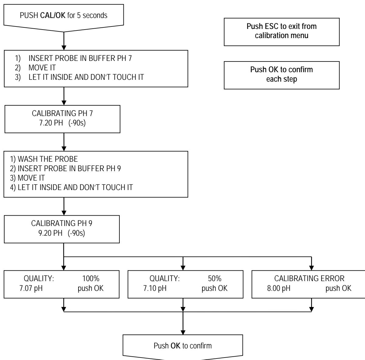
**NOTE:** After calibrating the electrode with the solution pH 9 the instrument could show the alarm concentration error, this alarm will disappear when the electrode is put into operation.
